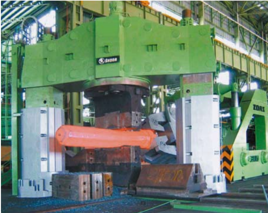
Forging unit with the CKW 6300 press and QKK 80 manipulator – Iran
