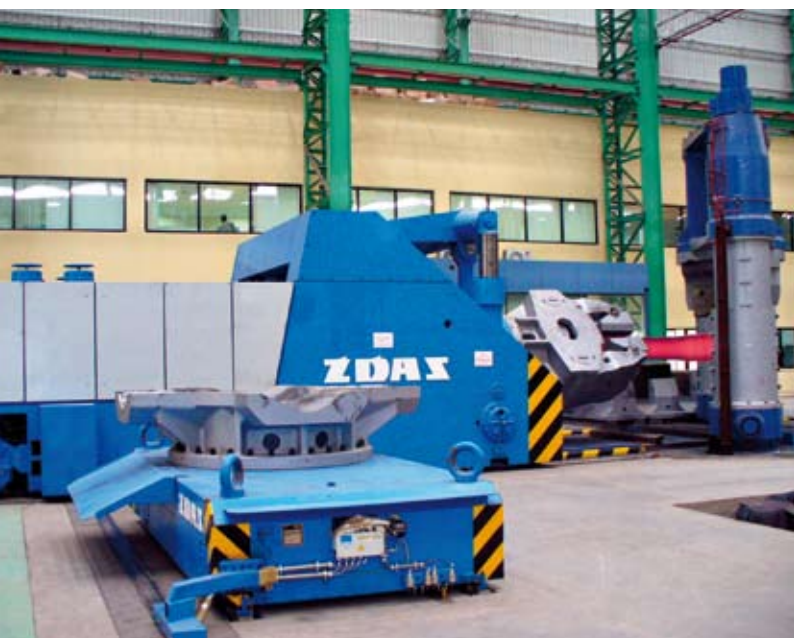
Forging manipulator QKK 35 and ingot bogie QHK 50, BFL, Pune, India
