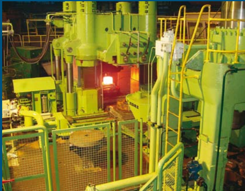
CKWZ 5600/6500 press – Bonatrans Bohumín, Czech Republic
