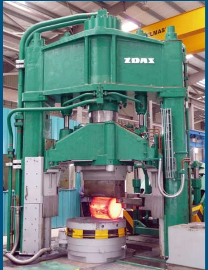
Forging unit with the press CKVX 1000 – Romania
